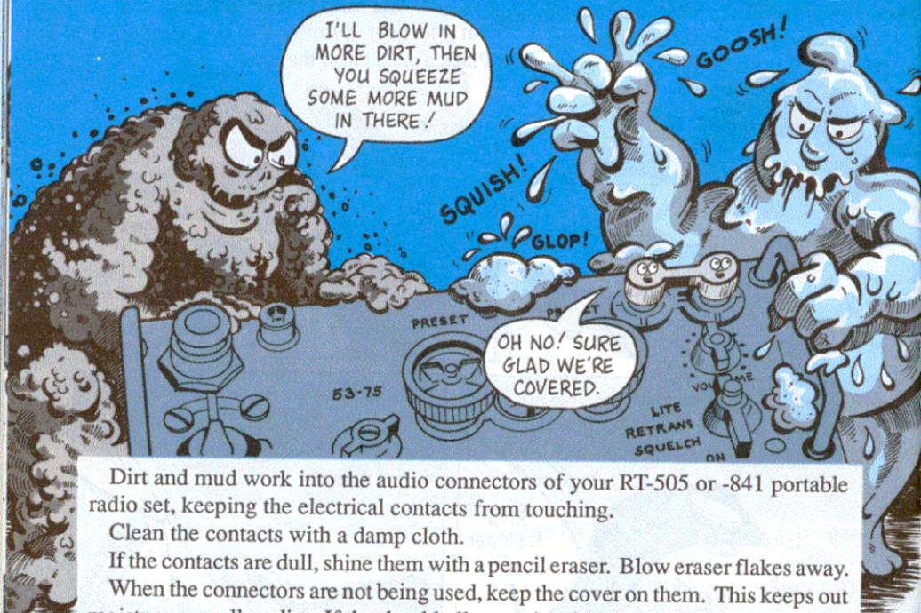
Dirt and mud work into the audio connectors of your RT-505 or -841 portable radio set, keeping the electrical contacts from touching.
