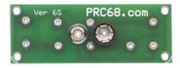
The two white lines are filing guides for rounding the two lower corners so that the adapter will fit the PSR-2. Version 6S printed circuit boards.
